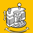
Centrifugal force adjustable from max. to min. by removing the lamellar weights.
