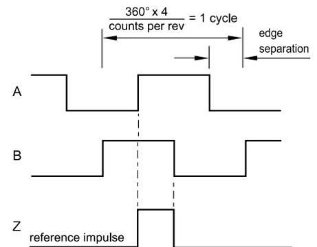
B leads A for clockwise rotation of magnetic actuator.
