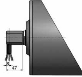
Cable slot 90° with threaded shaft
