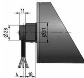
Elbow connector with shaft cap
