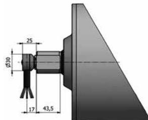
Elbow connector in stainless steel  $\leq 4,0$  kW
