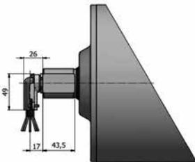
Elbow connector in aluminium  $\leq 4,0$  kW
