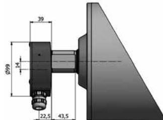
Terminal box in stainless steel  $\leq 4,0$  kW
