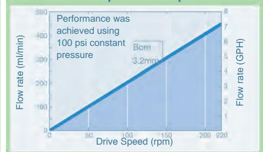
520 LoadSure® element pumpheads: flow ranges, 0.1-220 rpm, GPH\*
