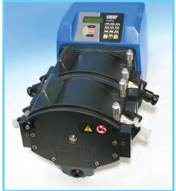
**Construction materials:** All 720 pumpheads are designed for strength and durability. Pumphead track: aluminum; drive shaft: stainless steel 440C; rotor end plates: aluminum; cradle assembly, track: aluminum; central shaft: EN24 steel; rollers: MOS2 filled Nylon 6 (Nylatron); springs, spindles: stainless steel; coating: Alocrom pre-treatment with polyester powder coating
