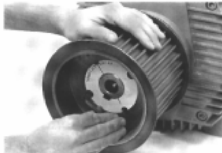
Step 4: tighten screws alternately
