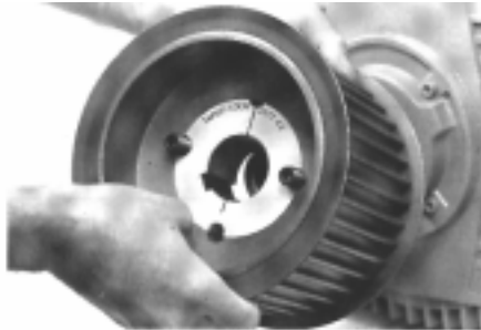
Step 2: insert screws and locate on shaft
