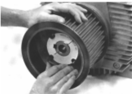
Step 3: tighten screws finger tight
