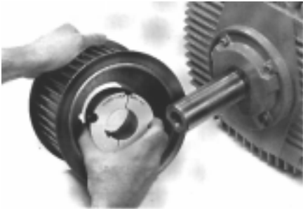
Step 1: insert bush into pulley
