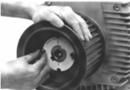
Step 3: tighten screws finger tight
