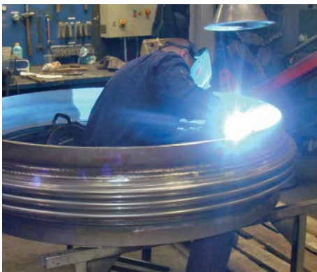
Welding a pipe end to a metal bellows.
