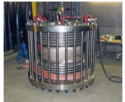
Testing a metal expansion joint with helium.
