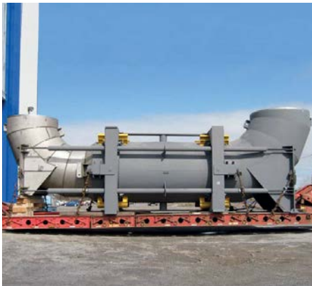
DN2300mm tied universal catalyst with slotted gimbals.
