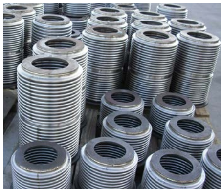
Metal pipe penetration seals.
