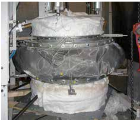
Low cycle fatigue test rig.
