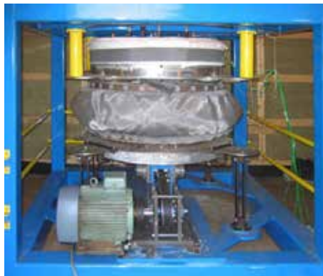
High cycle fatigue test rig.
