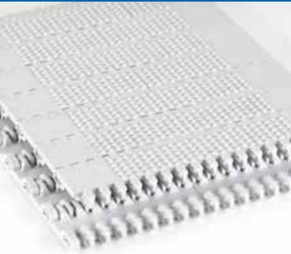
Textured top surface minimizes carry over waste through reduced product adhesion to the top surface.
