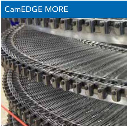
EDGE driven and cageless spiral conveyor belt in mesh overlay allows for greater product carrying capabilities with unique drive method.
