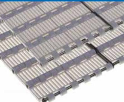
26% open area in small configuration to minimize product loss while draining. Stainless steel pins with reinforcing plates to minimize effect of thermal expansion at higher temperatures.
