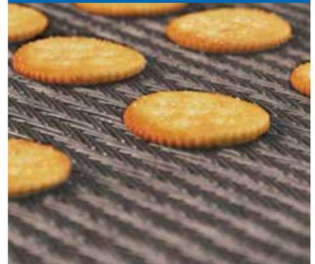
Our tighter mesh provides better tracking and baking than standard compound balance belts.
