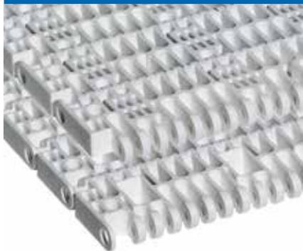
2.25" pitch heavy-duty design resists impact and abrasion with class-leading 45% open area to maximize water drainage.
