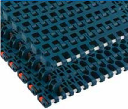
Increased performance, sustainability and safety. 1.2 turn radius and reinforced outer edge increases strength. Low friction RBT tab reduces friction for higher speeds.
