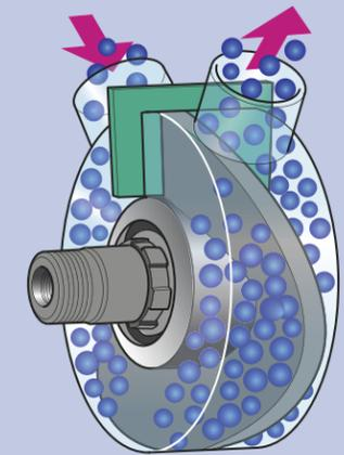
A single sinusoidal rotor in the pump creates four evenly sized chambers as it rotates within the pump. Fluid is “pulled” through the inlet on the suction side into each chamber in turn. As each chamber rotates, it contracts, closes and finally discharges fluid through the outlet port. At the same time, the opposite chamber opens to draw in more fluid. The result is a perfectly smooth flow, free of any pulsation.
